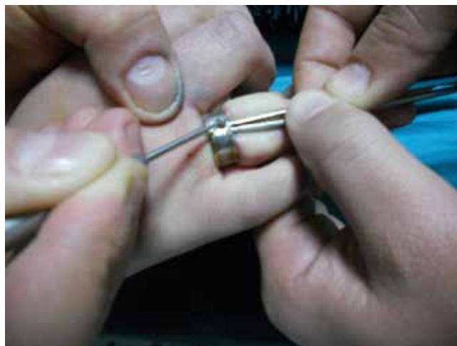
Figure 3. Cutting the ring with the high-speed motor.
